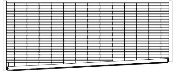
Standard grilles that require the use of a sloping bottom bar will use a traditional sloping bottom bar that includes a pitch plate.
