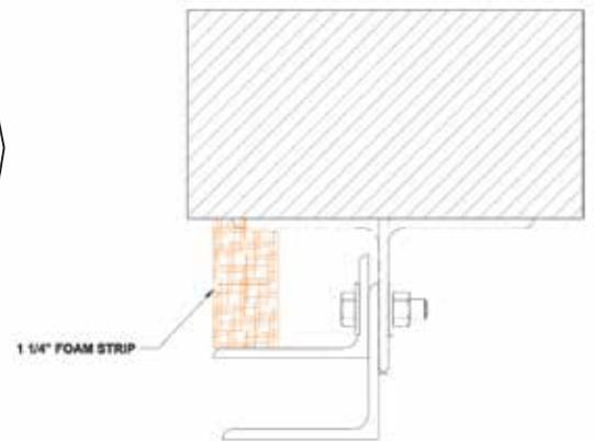
Air Infiltration value of less than .3 CFM/FT<sup>2</sup>.
