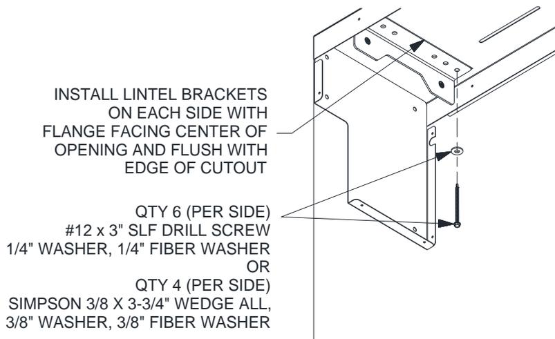
Figure 7.27 – Install 3 x 3 Tube on each side
