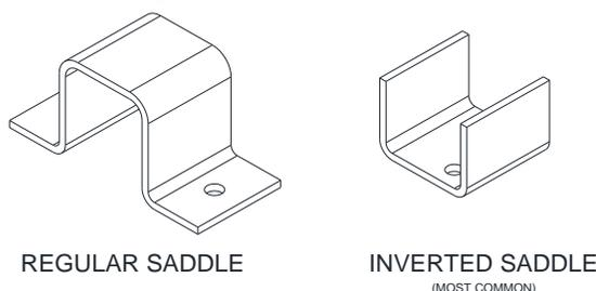
Figure 7.44 – Tube Saddle Hole location
