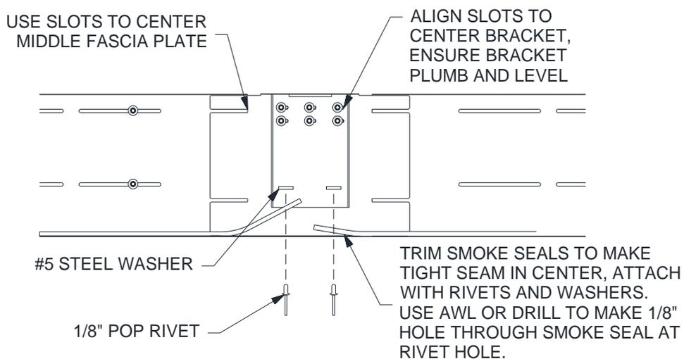
**Figure 7.5 – Upper Support Bracket attachment**
