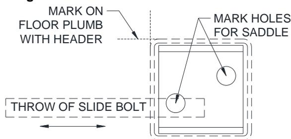
7. Use the mark placed on the floor in the previous steps, to locate where the saddle will be and mark the hole locations by placing the saddle on the floor. See **Figure 7.44**.
