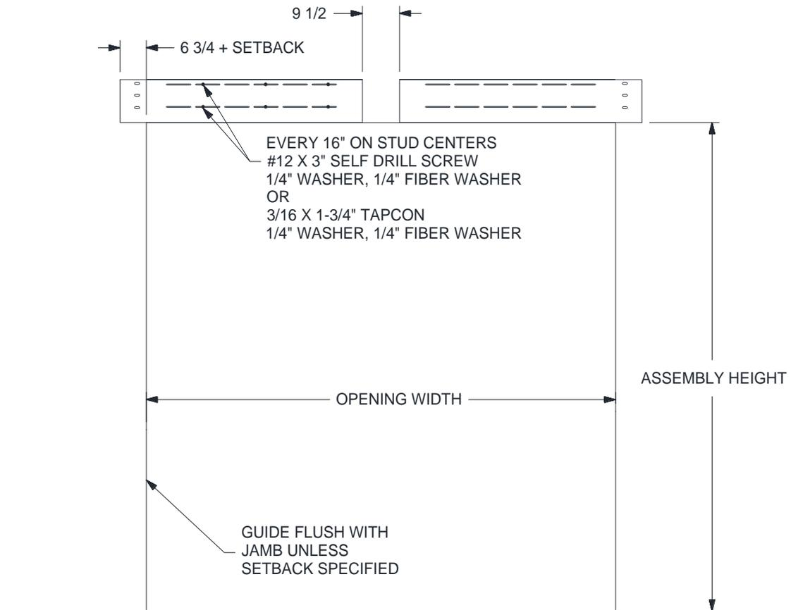
**Figure 7.2 – Fascia Hood Plate attachment – Isometric View**
