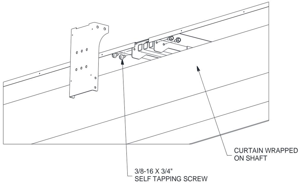
Figure 7.10 – Cross Brace Support Bracket attachment
