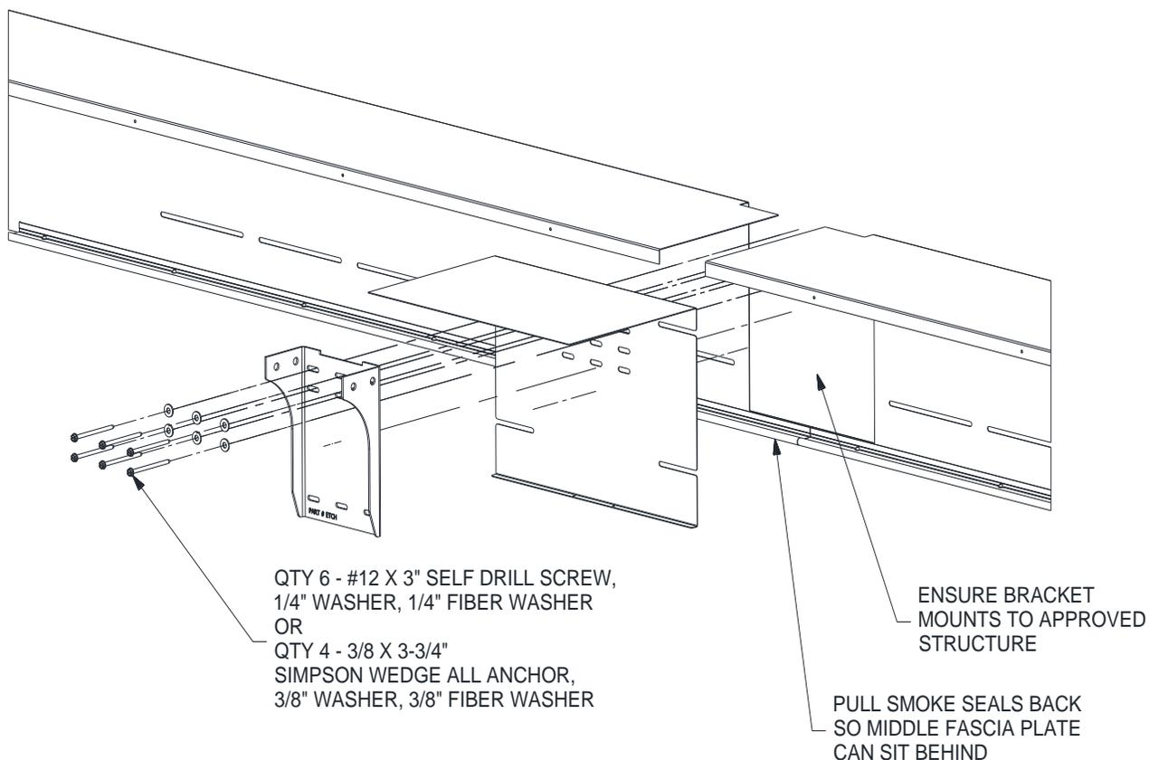
**Figure 7.4 – Middle Fascia Plate and Support Bracket Alignment**
