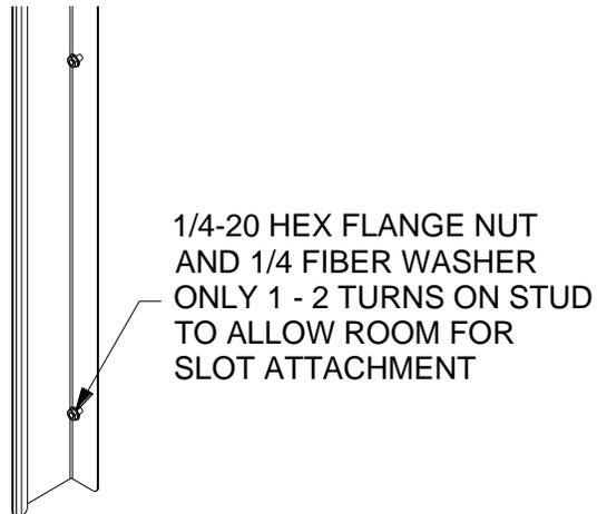
Figure 7.12 – Coil Side Guide attachment
