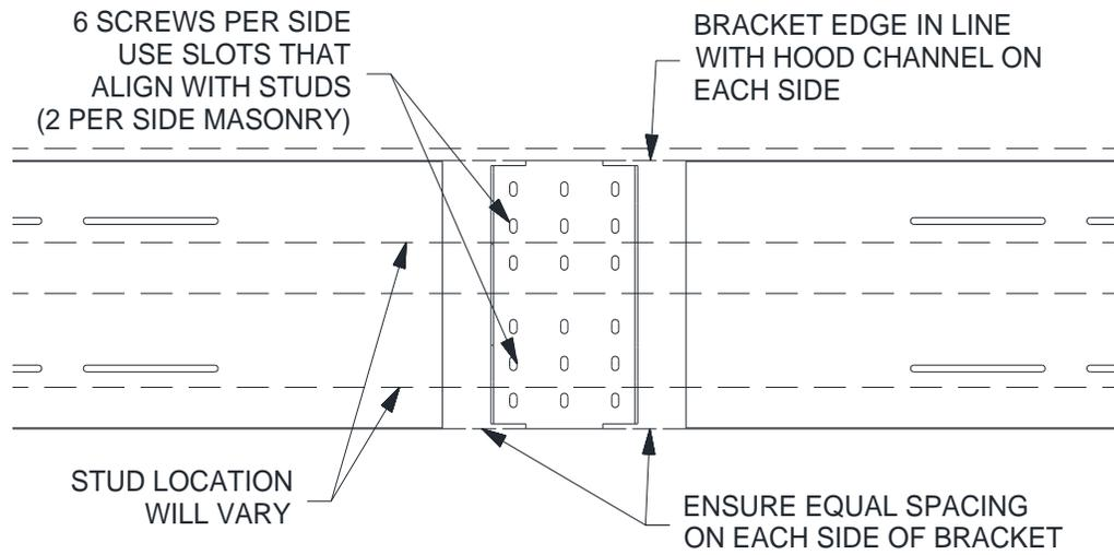
Figure 7.25 – Front Shaft Support attachment to Upper Shaft Support
