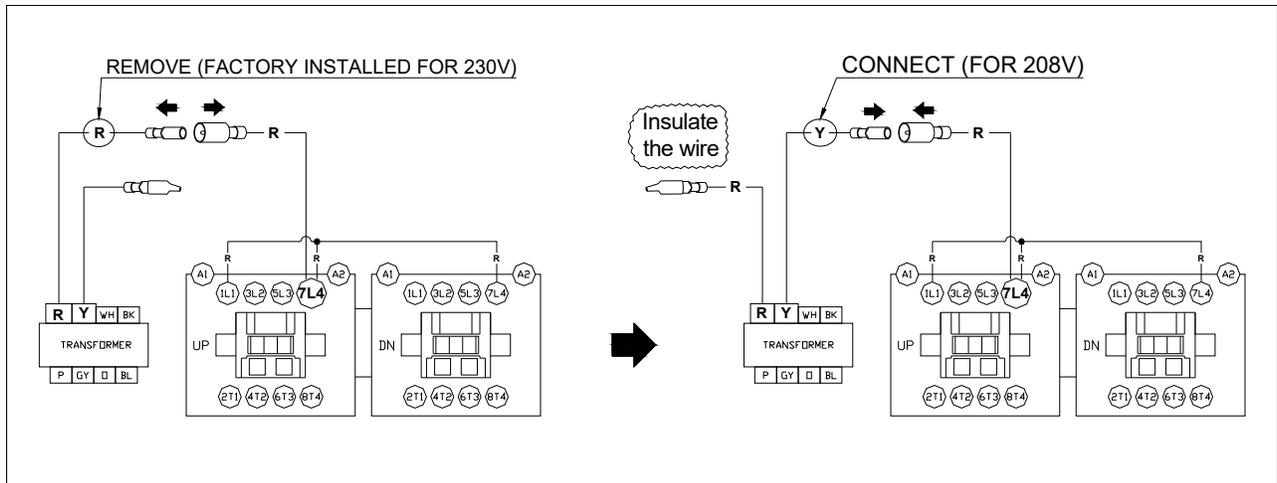
1. Unplug the red "230V" wire connector from the red "PWR" wire connector. Remove the insulating cap from the yellow "208V" wire connector.
