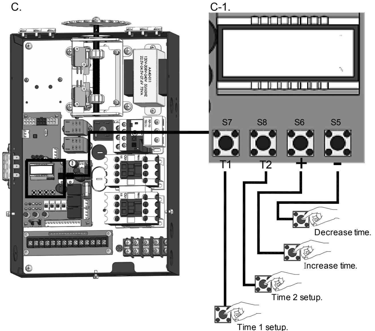
(1) Timer 1 – Mid-open timer: Timer starts counting when door leaves close limit. Door stops after opening for set time. Pressing open again at mid-open position will cause door to open limit.
