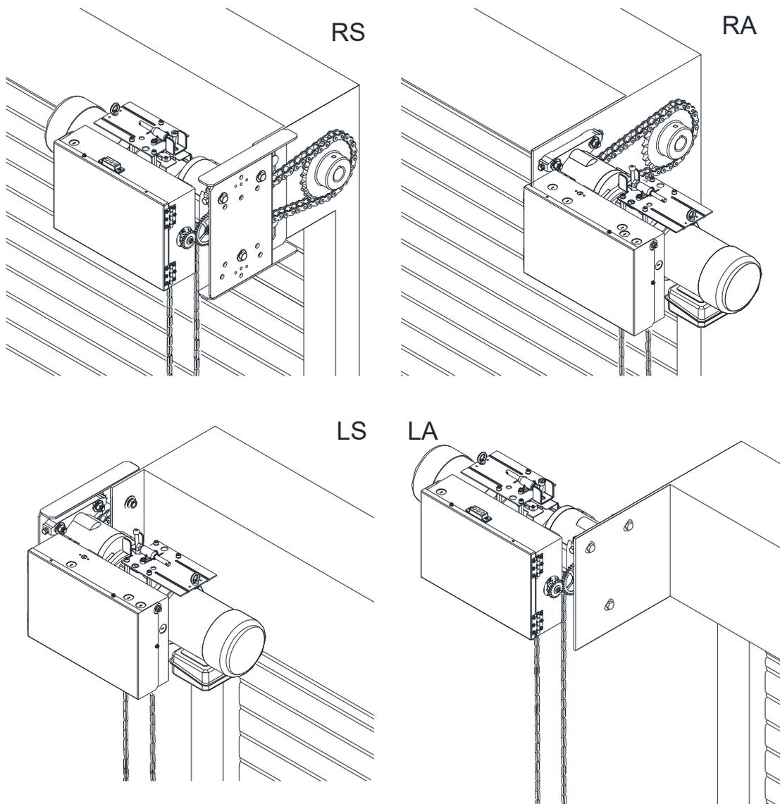
Installation positions for larger horsepower units are similar to as shown above.
