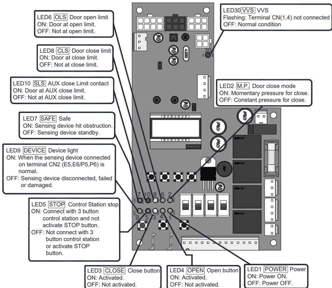
FGH 230V 1 PHASE 50HZ LH (FGEP BOARD)
