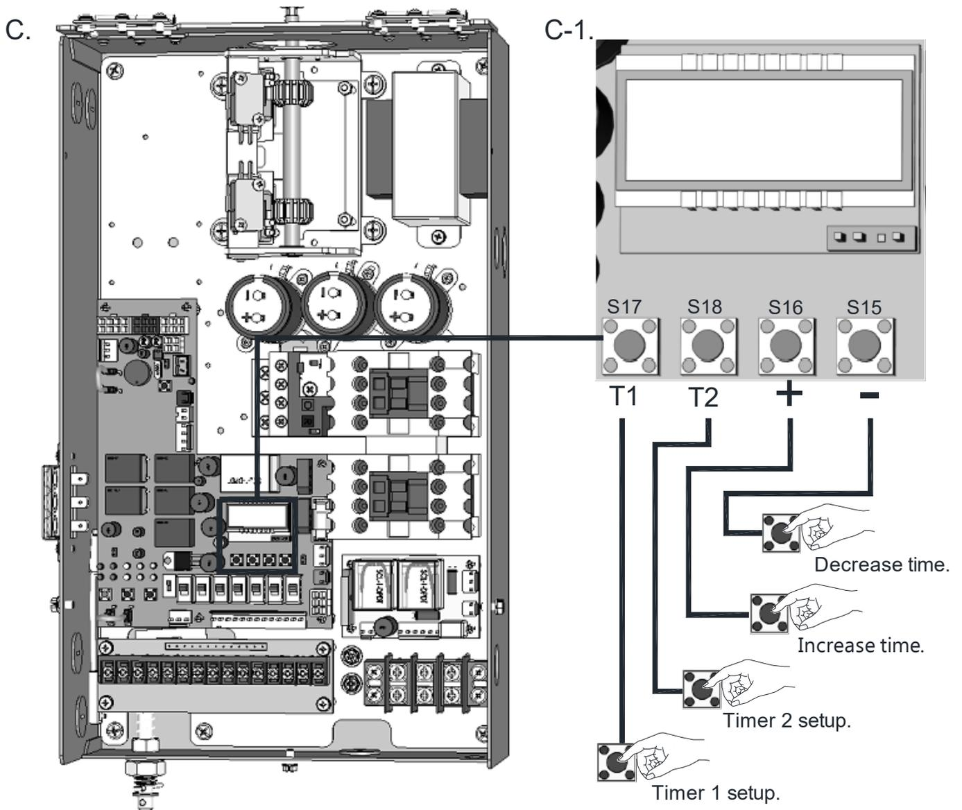
1. Time 1 – Mid-open timer : Timer starts counting when door leaves close limit. Door stops after opening for set time. Pressing open again at mid-open position will cause door to open limit.
