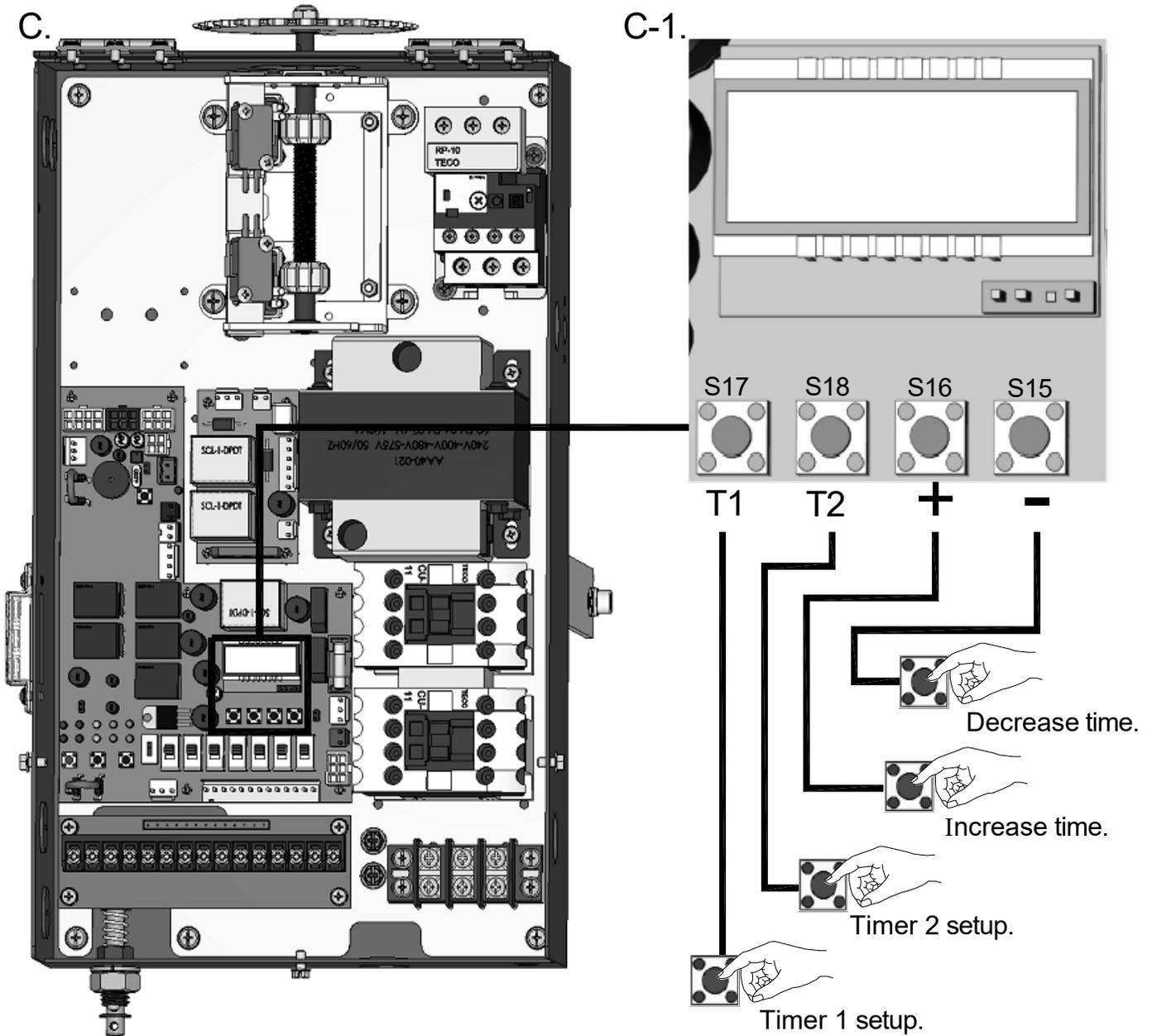
(1) Timer 1 – Mid-open timer: Timer starts counting when door leaves close limit. Door stops after opening for set time. Pressing open again at mid-open position will cause door to open limit.
