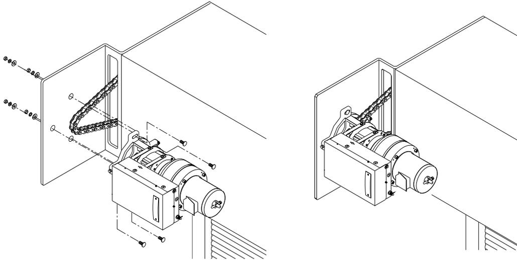
4. When the operator assembly is attached to the door bracket, be sure the door driven sprocket is properly aligned with the operator drive sprocket before securing the driven sprocket to the shaft.
