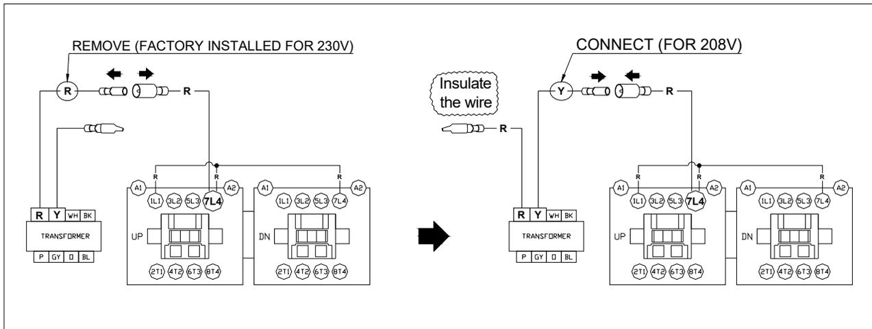
1. Unplug the red "230V" wire connector from the red "PWR" wire connector.
