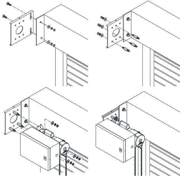
6. When the operator assembly is attached to the door bracket, be sure the door driven sprocket is properly aligned with the operator drive sprocket before securing the driven sprocket to the shaft.
