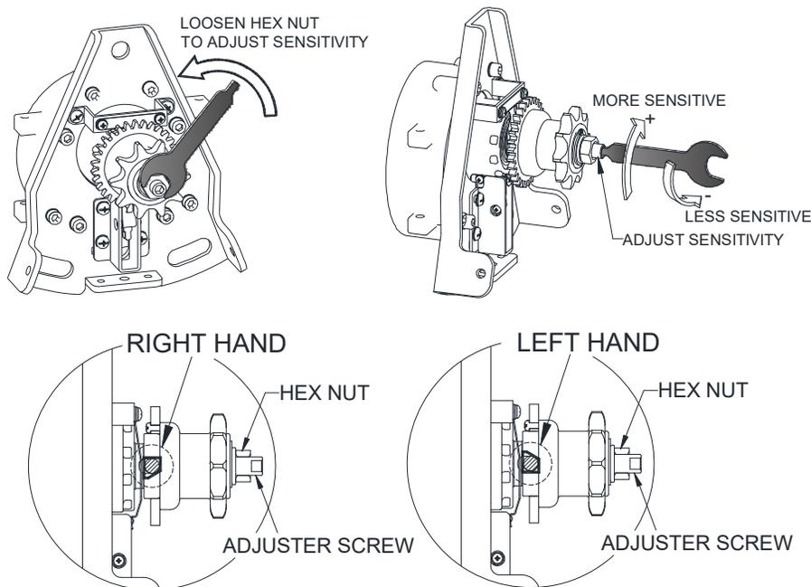
**NOTE:** 6 turns of the lock sensor adjustment will result in the lock sensor in the least possible sensitivity, which means the greatest amount of pull against the locking device. If the door is still not functioning properly, check spring tension, overall door installation and consult door manufacturer.
