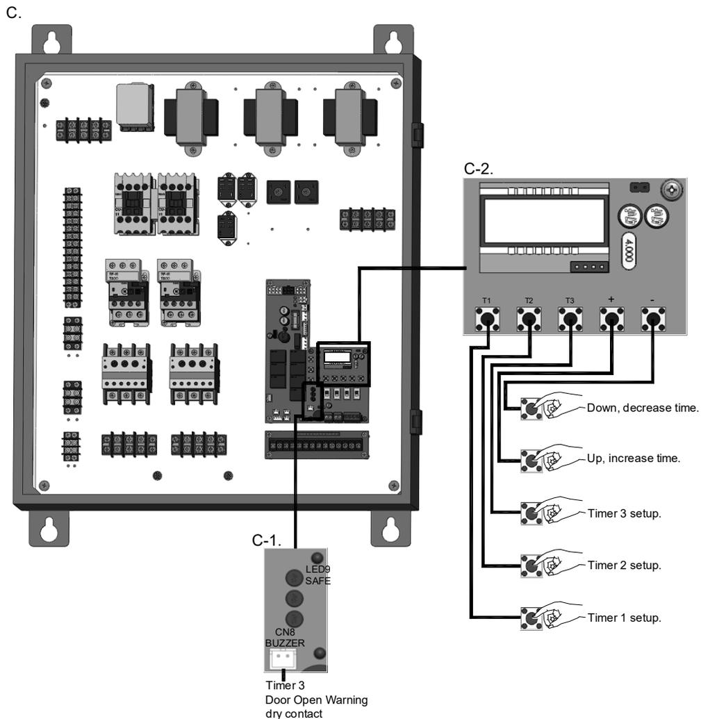
(1) T1 – Mid-open timer : Timer starts counting when door leaves close limit. Door stops after opening for set time. Pressing open again at mid-open position will cause door to open to open limit.
