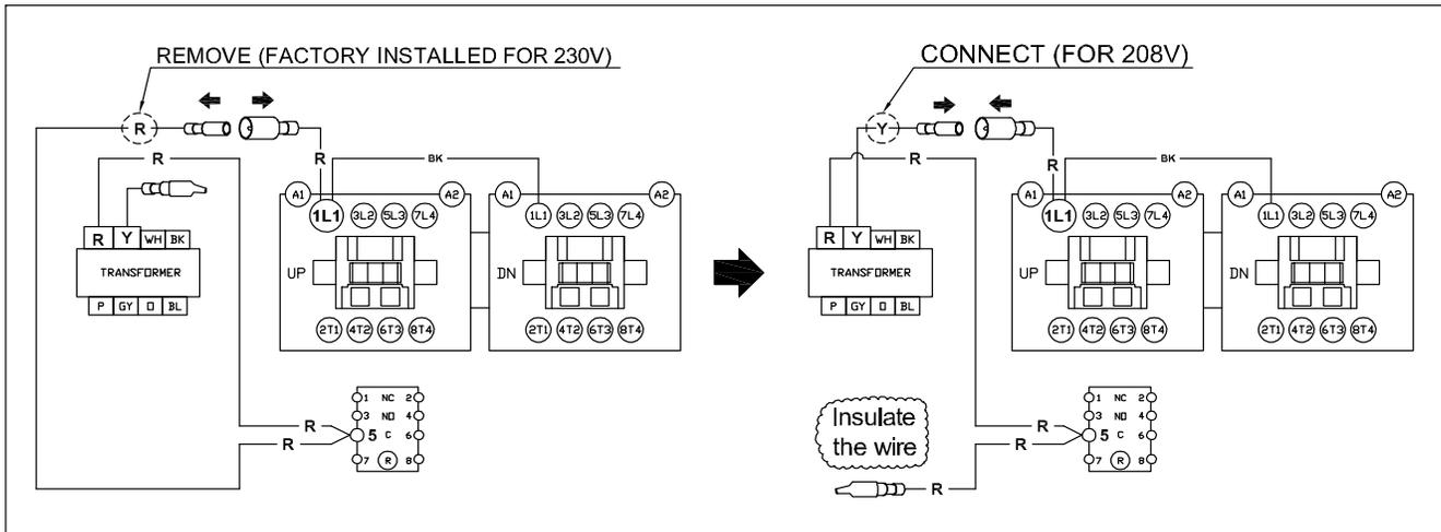
1. Unplug the red "230V" wire connector from the red "PWR" wire connector. Remove the insulating cap from the yellow "208V" wire connector.
