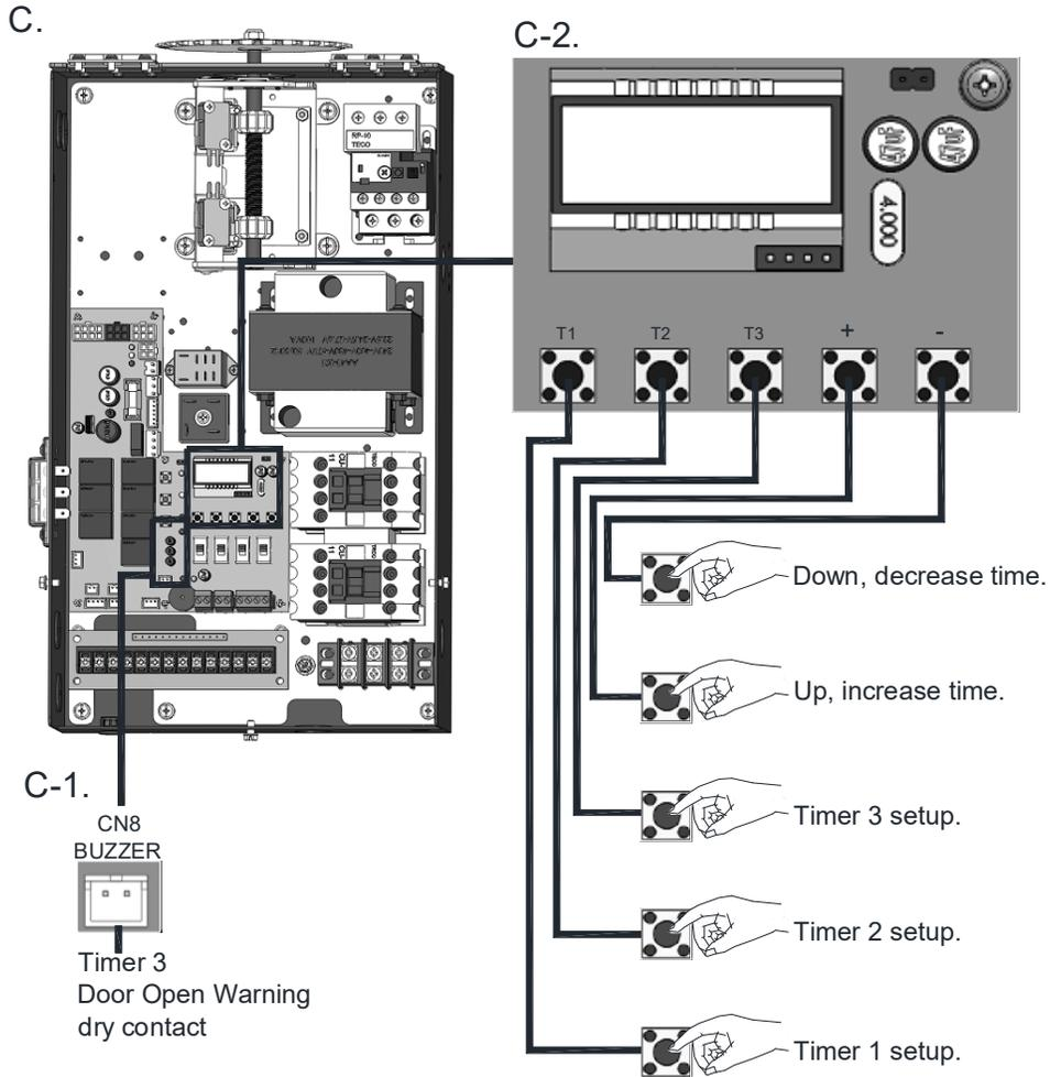
1. T1 – Mid-open timer : Timer starts counting when door leaves close limit. Door stops after opening for set time. Pressing open again at mid-open position will cause door to open to open limit.
