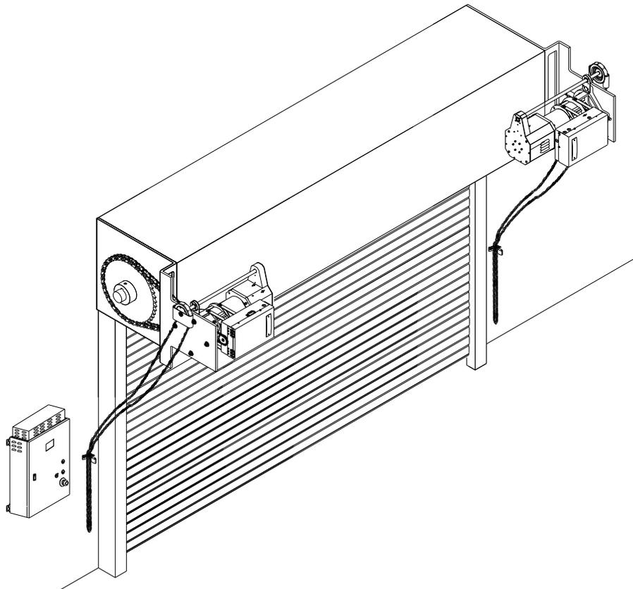
6. When the operator assembly is attached to the door bracket, be sure the door driven sprocket is properly aligned with the operator drive sprocket before securing the driven sprocket to the shaft.
