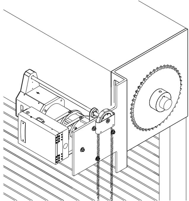
3. After mounting on operator at each side and before putting on the roller chain, checking the motor Rotation directions if both motors are correct through push the OPEN or CLOSE buttons.
