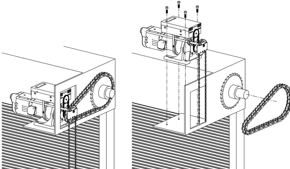
1. When the operator assembly is attached to the door bracket, be sure the door driven sprocket is properly aligned with the operator drive sprocket before securing the driven sprocket to the shaft.
