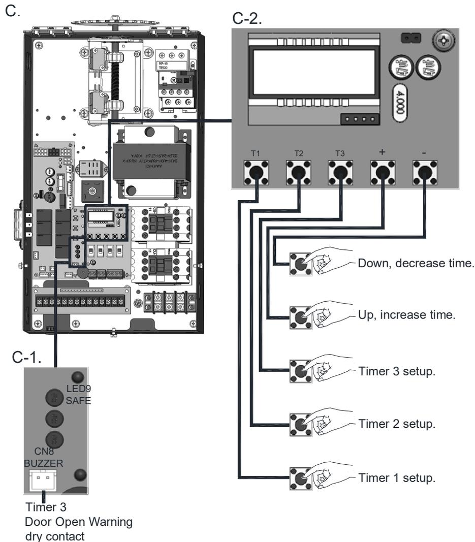
(1) T1 – Mid-open timer : Timer starts counting when door leaves close limit. Door stops after opening for set time. Pressing open again at mid-open position will cause door to open to open limit.
