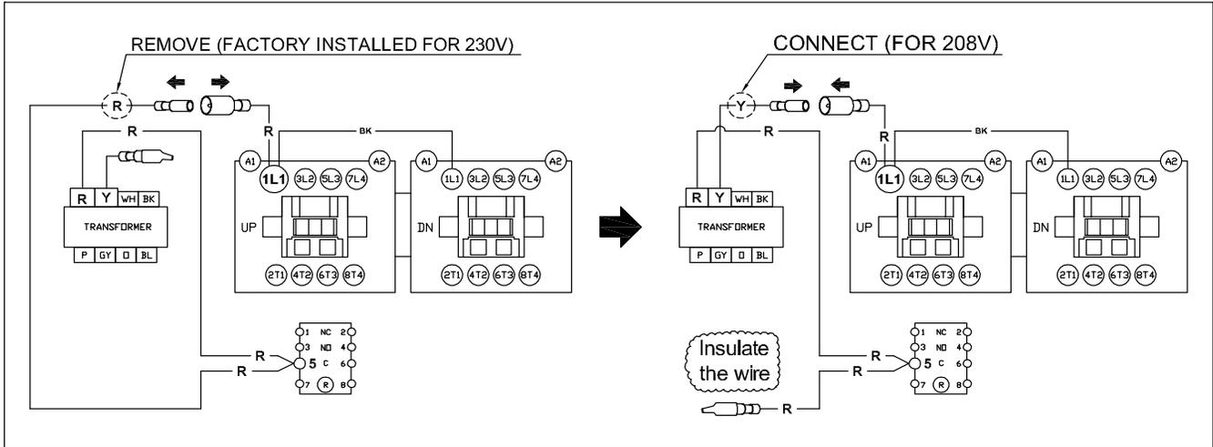
1. Unplug the red "230V" wire connector from the red "PWR" wire connector.
