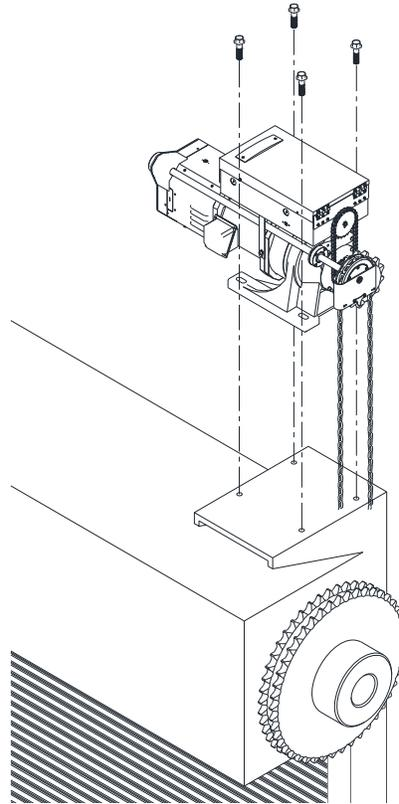
3. After mounting on operator at each side and before putting on the roller chain, checking the motor Rotation directions if both motors are correct through push the OPEN or CLOSE buttons.
