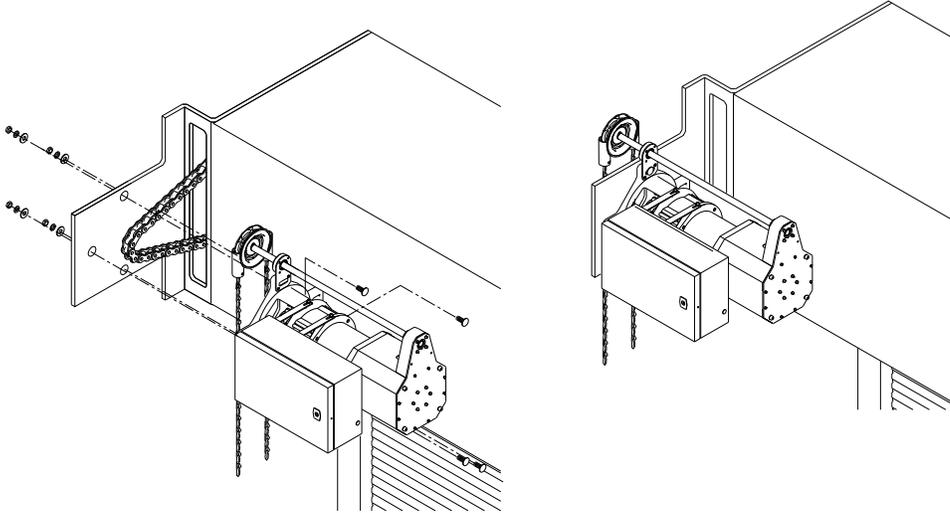
4. When the operator assembly is attached to the door bracket, be sure the door driven sprocket is properly aligned with the operator drive sprocket before securing the driven sprocket to the shaft.
